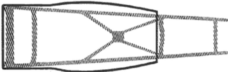
Above—Black line shows how body is mounted to frame in ordinary car. Note overhang.
